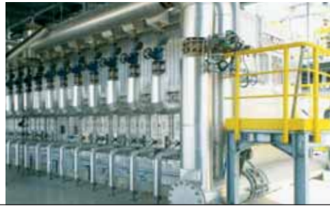
The GEA Niro CONTACT FLUIDIZER™ fluid bed utilizes heating panels submerged in the fluidized product layer, which provides energy savings of 10-25% depending on product type and grade.
