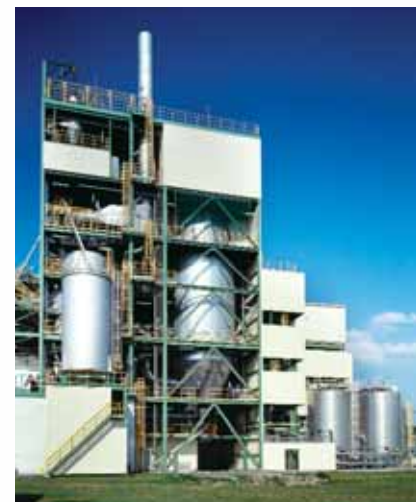
The NOZZLE TOWER™ spray dryer enables production of extra-fine grade e-PVC powder.
