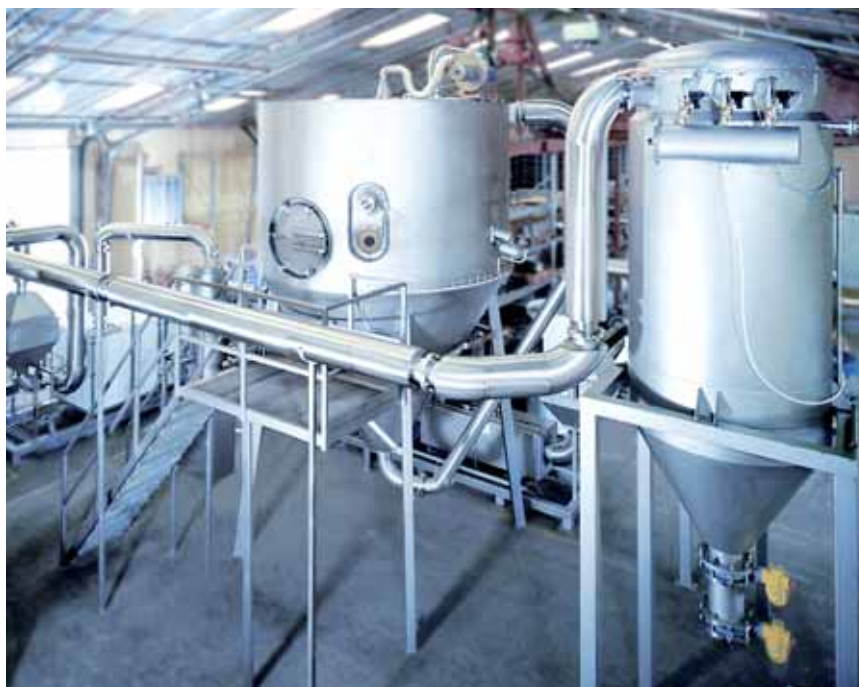
VSD-12.5-CC spray dryer with a rotary atomizer. Closed-cycle design using nitrogen as drying gas. Drying chamber size: Ø 2500x2000 mm, 60° cone.
