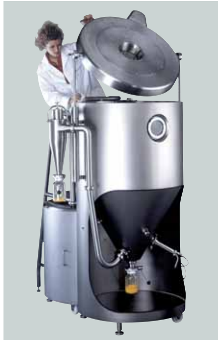
The MOBILE MINOR™ version with pneumatically liftable chamber roof. Here equipped with fountain two-fluid nozzle and two-point powder collection. Drying chamber size: Ø 800x620 mm, 60° cone.
