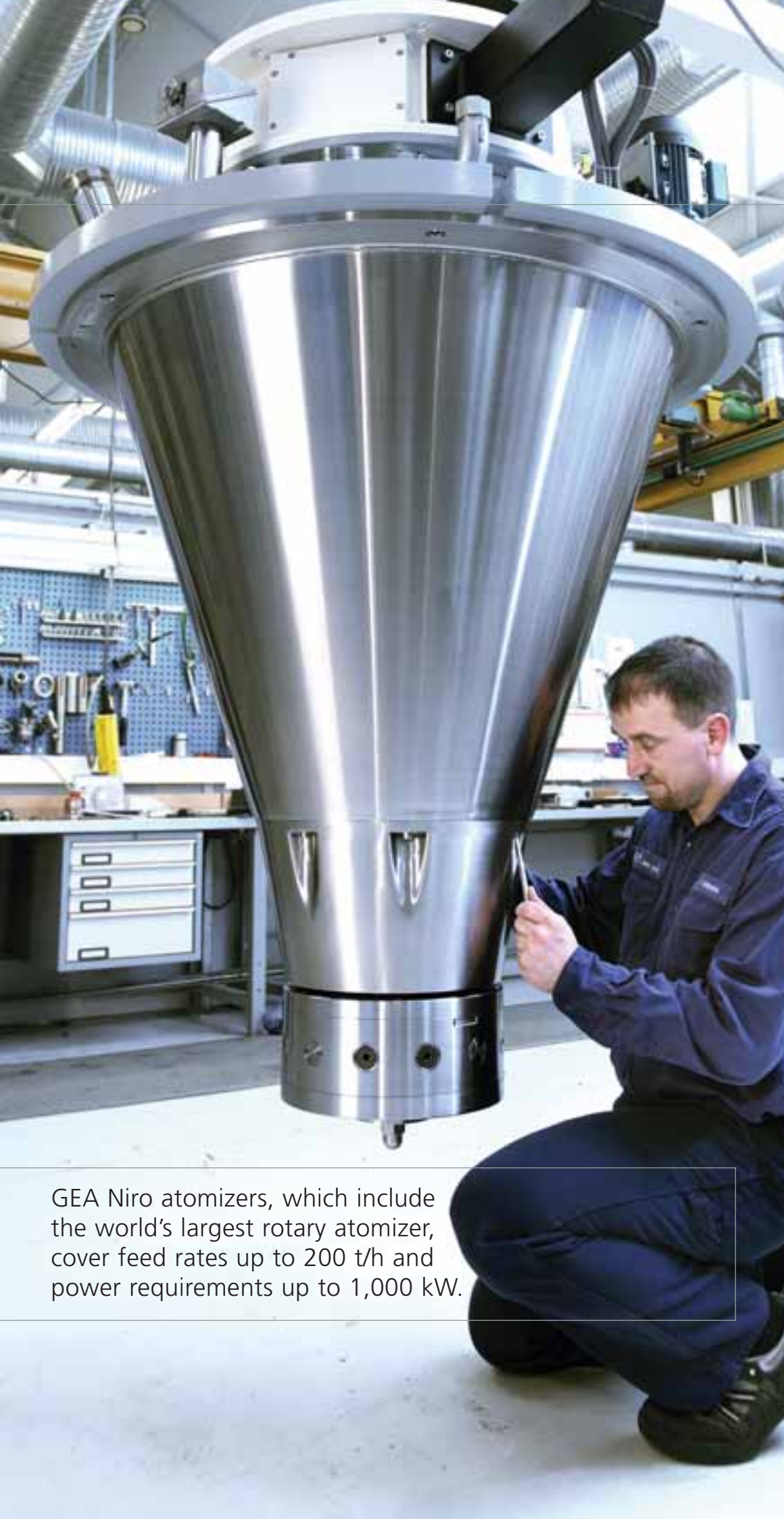
Rotary atomizer (top) and nozzle atomizer sprays
