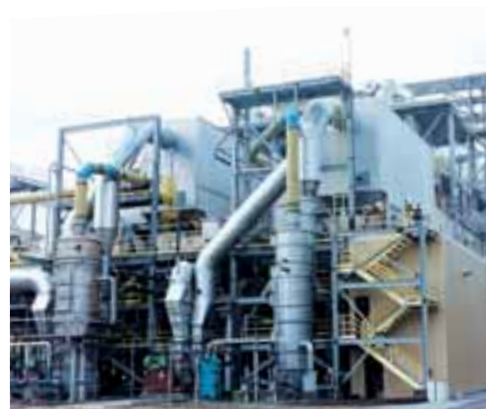
GEA Niro CONTACT FLUIDIZER™ with integrated filters for the production of dense soda ash
