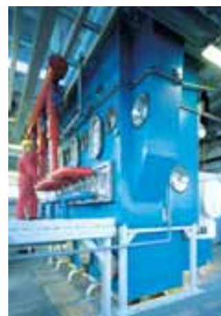
GEA Niro SPRAY FLUIDIZER™ plant for the production of granulated food preservatives
